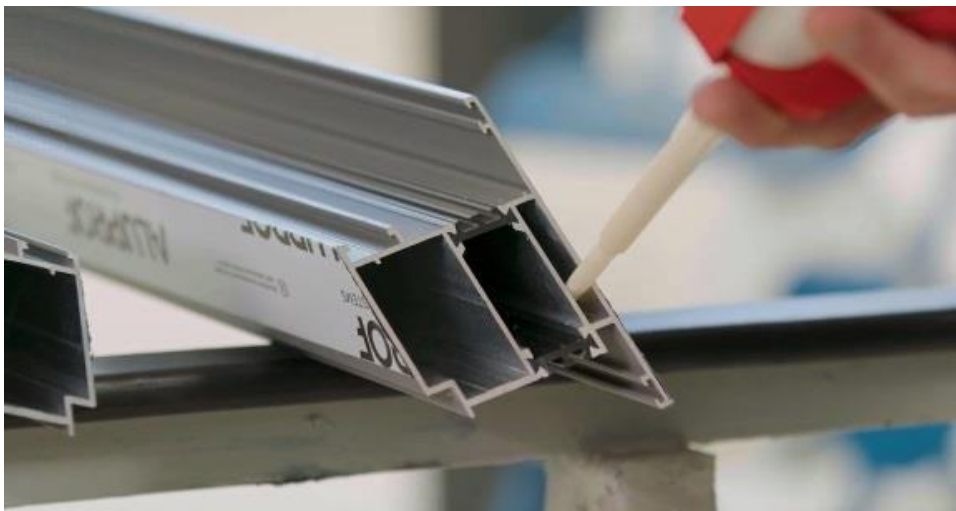
Applying glue to the profile chambers
