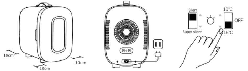
**Step1.**Keep a 10cm distance around the product, Make sure there is no plug in the air inlet cooling hole.
