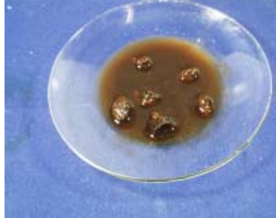
F4: Seriously damaged fluid, residues non-redissolvable
