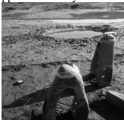
Fig. 2. Explosive loading of worn excavator bucket teeth (Drahobetskyi, Shapoval, Shchepetov et al., 2017)
