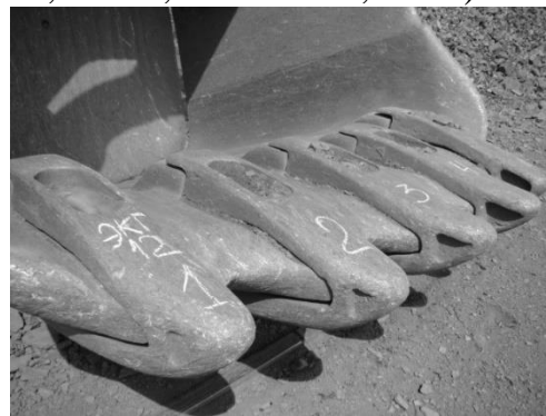
Fig. 8. Appearance of worn teeth (Drahobetskyi, Shapoval, Shchepetov et al., 2017)
