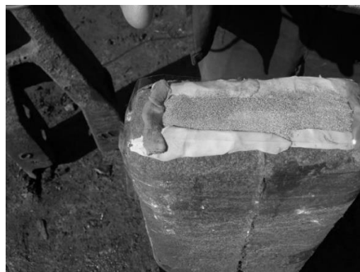
Fig. 4. Tooth tip with Ti+V powder (titanium + vanadium) (Drahobetskyi, Shapoval, Shchepetov et al., 2017)
