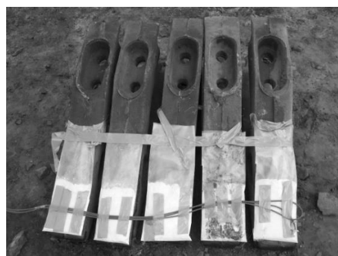
Fig. 6. Hardening scheme with explosive wave (Drahobetskyi, Shapoval, Shchepetov et al., 2017)
