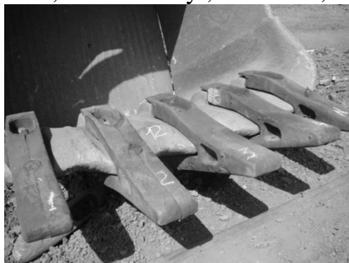
Fig. 7. Hardened teeth on the excavator bucket (Drahobetskyi, Shapoval, Shchepetov et al., 2017)
