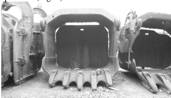
Fig. 1 – Worn buckets of quarry excavators (Drahobetskyi, Shapoval, Shchepetov et al., 2017)
