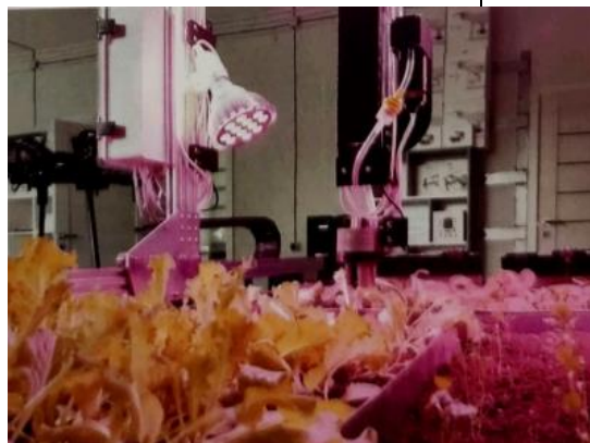
The agrorobot takes care of the plants in FarmBot installation
